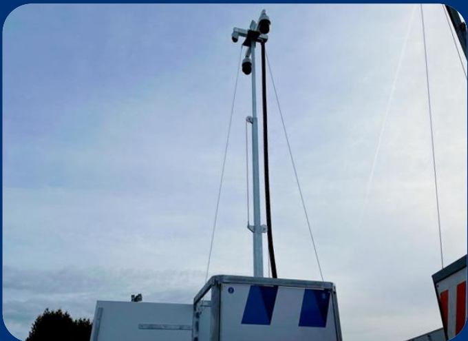
6. Extend the mast fully until the guy wires are taut. Please note: do not turn it with excessive force!
