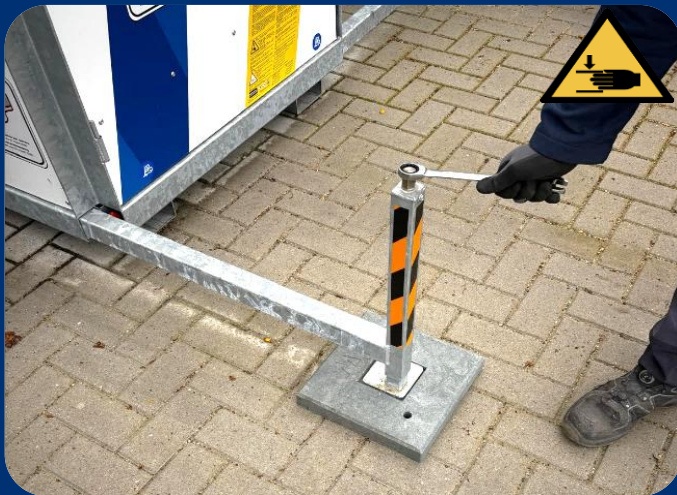
3. Pull the support legs out and place a tile underneath. Use the 19 mm spanner to unscrew the legs. Use this to level the tower.
