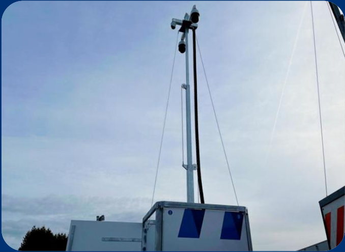
7. Extend the mast fully until the guy wires are taut. Please note: do not turn it with excessive force!
