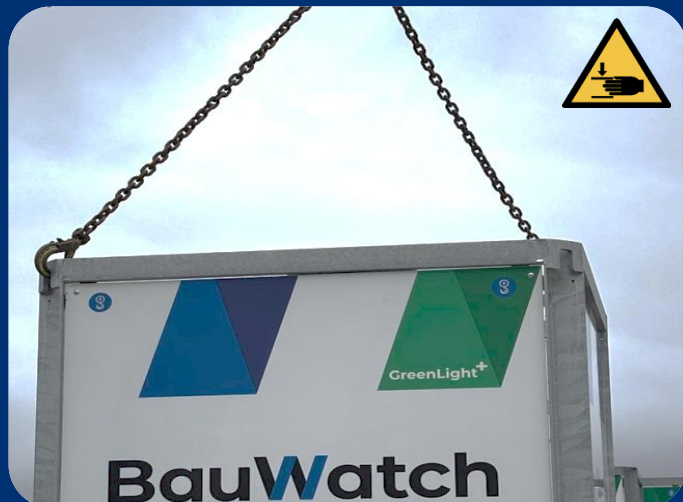
3. Use an approved lifting chain (minimum 2-leg) crosswise to hoist the tower. Use the hoist-eyes.
