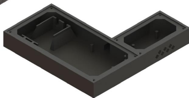
Case re-designed for AM – printed using Carbon PEEK in one monolithic piece, no assembly required
