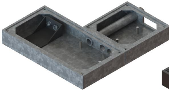
Autoclave case manufactured with traditional method – 15 parts, long assembly
