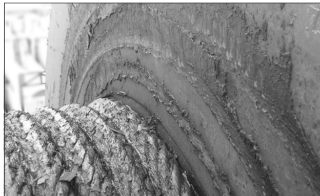
Fig.: Wear on a drum flange
