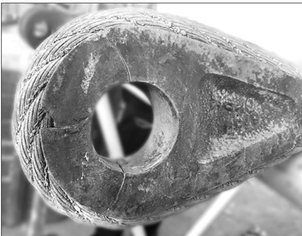
Fig.: Cracks in a solid thimble
