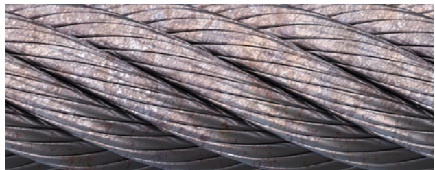
Fig.: Slight corrosion, 0% - 20% severity
