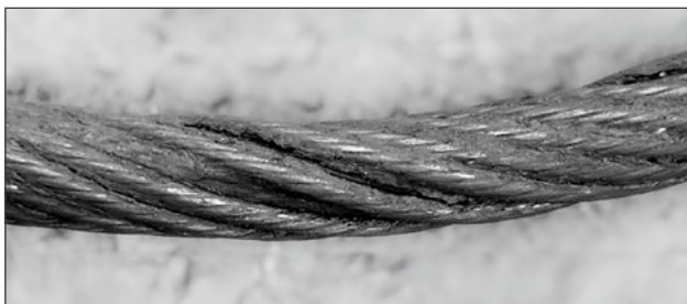
Fig.: Local decrease of rope diameter
