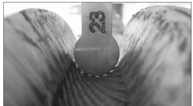
Fig.: Clearly visible impressions of a negative rope profile
