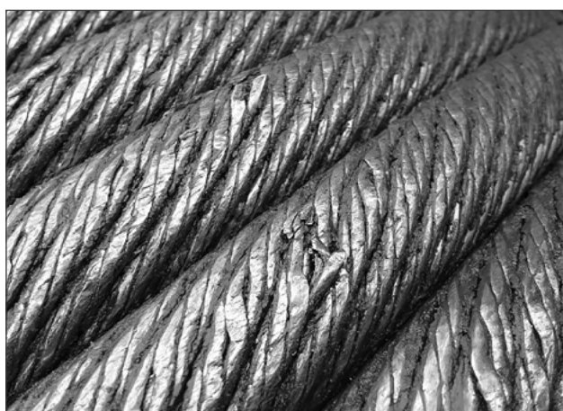
Fig.: Wear in multi-layer spooling
