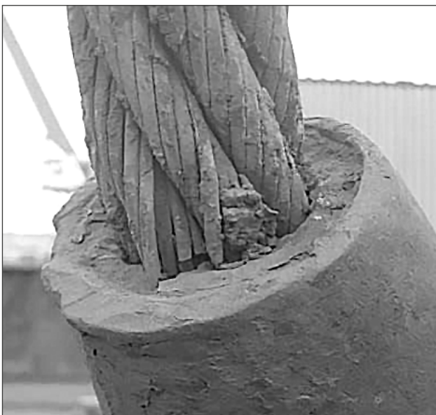
Fig. 3: Wire breaks at rope end termination
