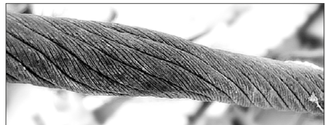
Fig.: Flattened portion
