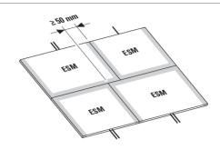
3) Install the sensor with the type plate facing down. The grip pads should always be on the top side.
