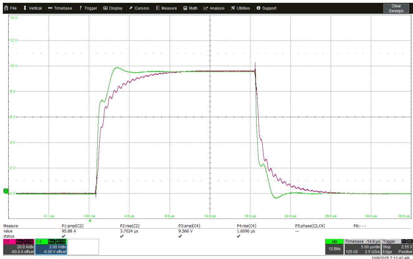
**I-Mon Transient Response**, DUT: CMD-100: CH2: Reference Current (Shunt), CH4: I-Mon,  $t_{PW}=20 \mu s$ , Gain=0.1 V/A, Load:  $1 \Omega$ , Source: FIS 100-200 (Power Switch),  $U_{IN}=100 V$
