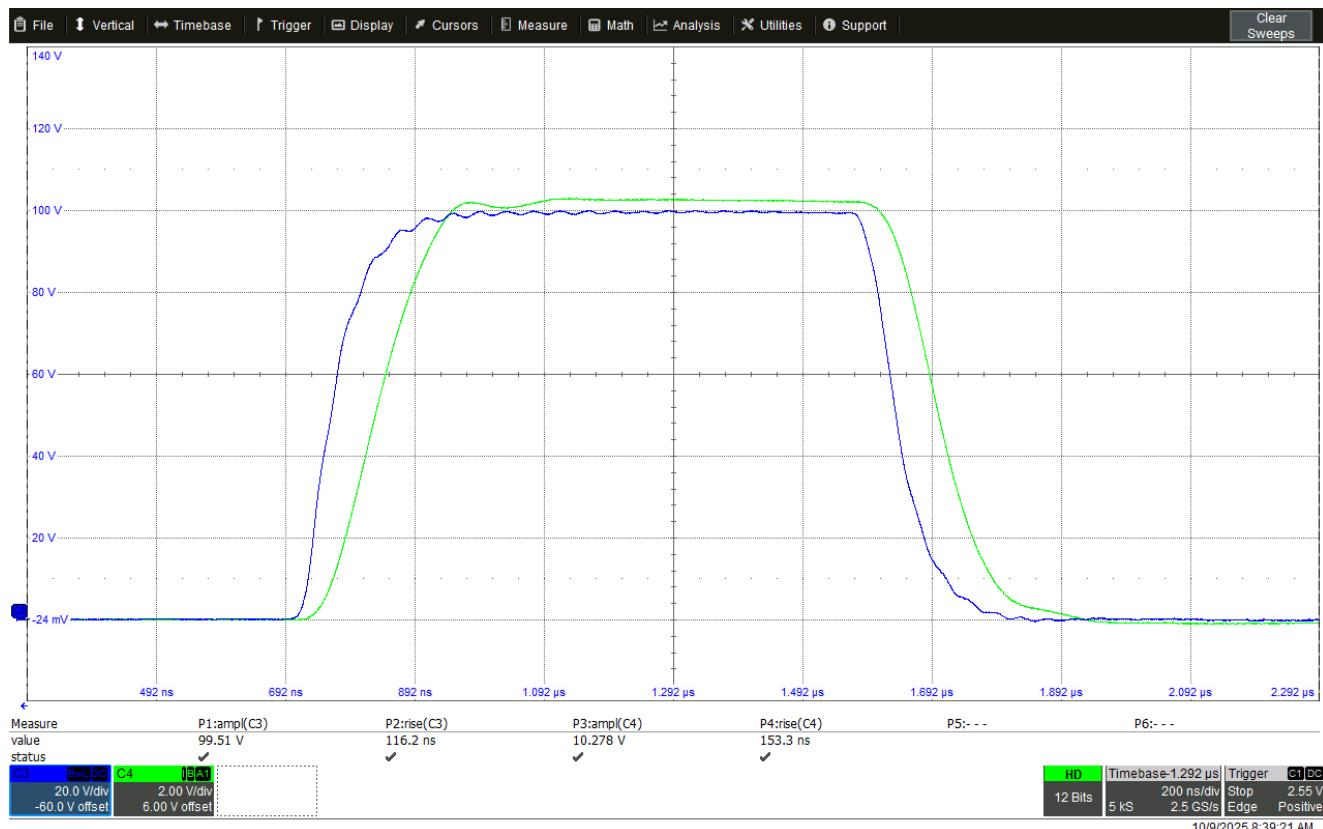
**U-Mon Transient Response**, CMD-100: CH3: Reference Voltage (Load), CH4: U-Mon (Load),  $t_{PW}=1 \mu s$ , Gain=0.1 V/V, Load: 1 kΩ, Source: FIS 100-200 (Power Switch),  $U_{IN}=100 \text{ V}$
