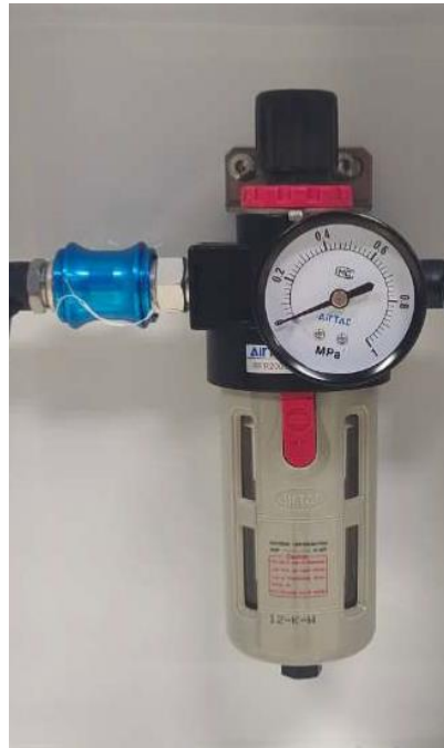
Figure 5-3 Connect air source to the equipment
