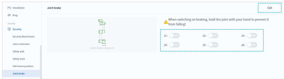
Figure 1.1 Manually release the brakes
