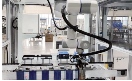
Battery Inspection Loading & Unloading
