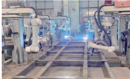
Steel Frame Welding
