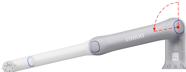
Figure 3.9 J2 Emergency stop test
