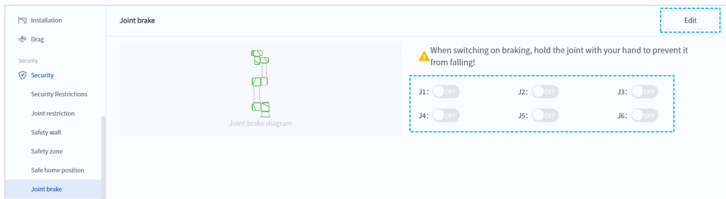
Figure 1.1 Manually release the brakes
