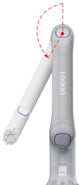
Figure 3.10 J3 Emergency stop test
