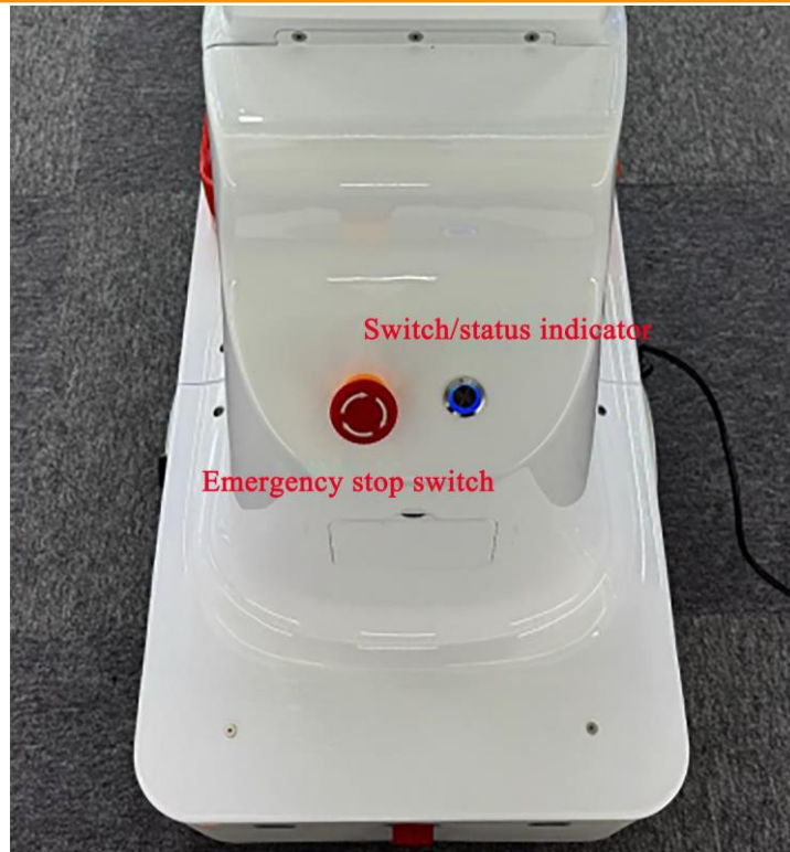
Fig. 6 Emergency Stop Switch and Switch/status Indicator Light
