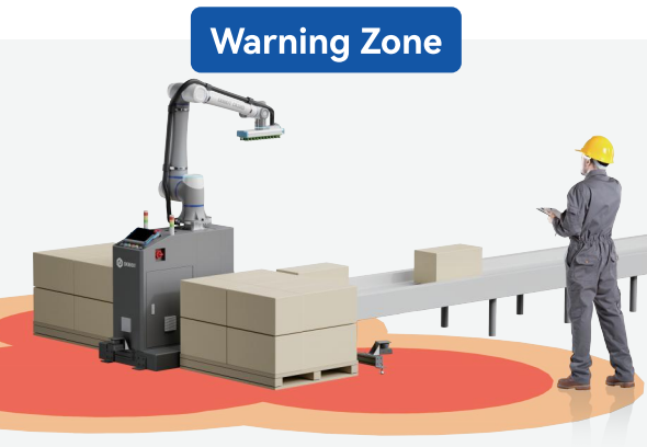
The robot operates at reduced speed, creating necessary margin for emergency avoidance.
