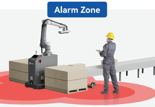
Triggers an immediate robot stop to prevent direct human-robot collisions.
