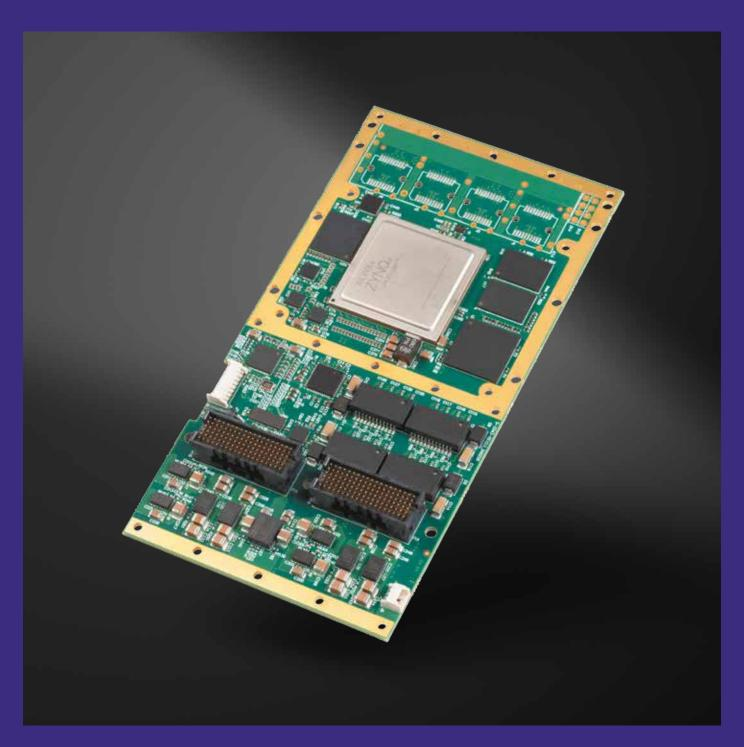
Time-Sensitive Networking Endpoint Switch XMC Mezzanine
