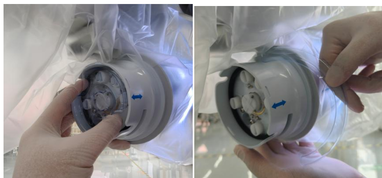
Figure 11 Remove the clamp and zero-position holder
