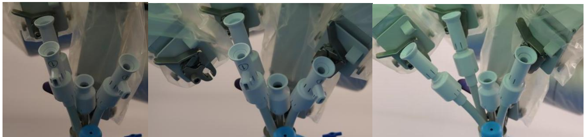
Figure 16 Adjust robotic arm 2, 1 and 4 successively, and connect instrument channel 2, 1 and 4
