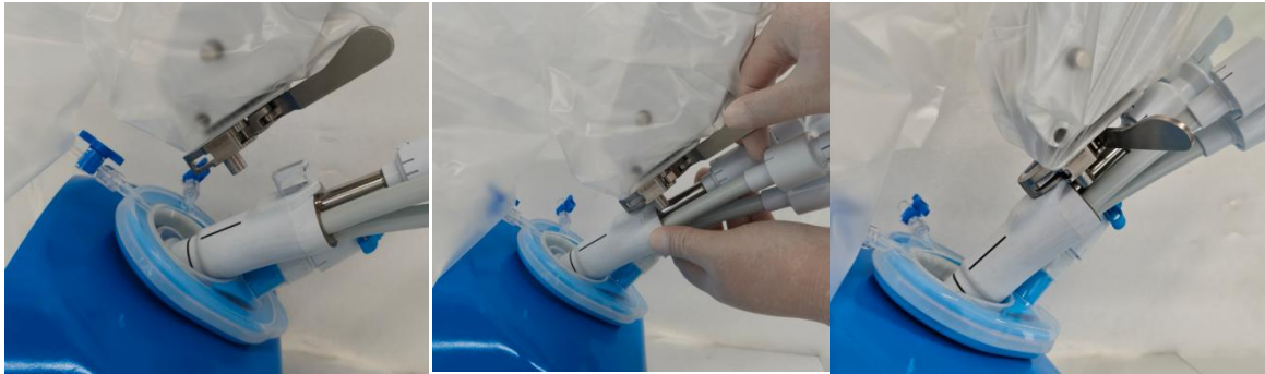
Figure 15 Connect robotic arm 3 of the Surgical Trolley to the 3D endoscope channel
