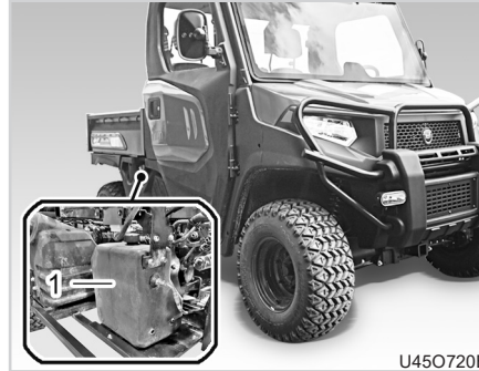
(1) Hydraulic Oil Tank
