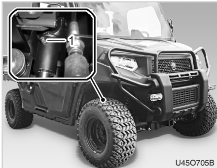
(1) Grease Fitting (Front axle drive shaft around gear box)
