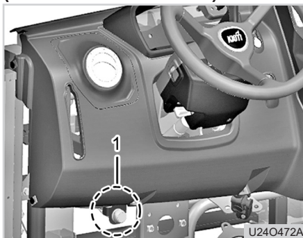
(1) Emergency start switch
