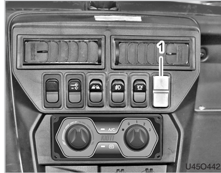
(1) Spare Switch Panel
