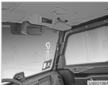
(1) Emergency Exit Label
