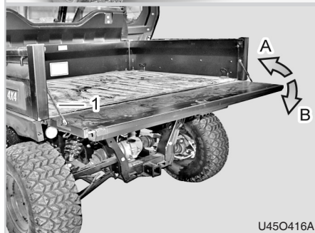
(1) Wire Rope (2) Door (3) Latch Handle (A) Close (B) Open
