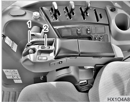
(1) Position Lever (2) One-touch Switch
