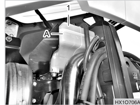
(1) Reservoir Tank (A) Min (Lack)
