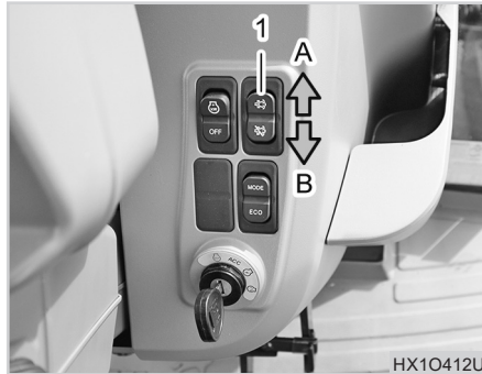
(1) DPF Regeneration Switch (A) Activation (B) Deactivation
