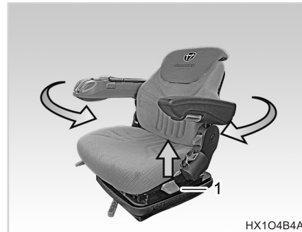
(1) Rotation Adjustment Lever
