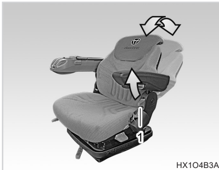
(1) Seat Back Adjustment Lever
