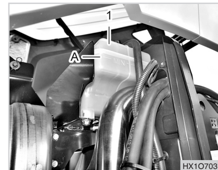
(1) Reservoir Tank (A) MIN (Lack)
