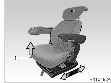
(1) Seat Adjustment Lever
