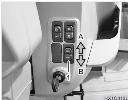
(1) ECO/MODE selection switch (A) MODE button (B) ECO button
