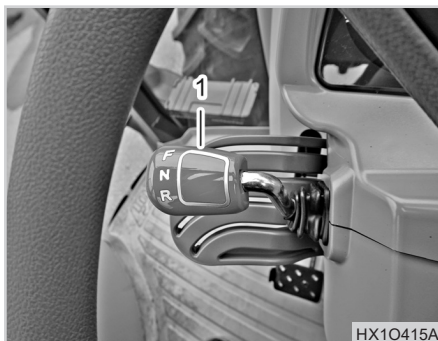
(1) Shuttle Shift Lever (F) Forward (N) Neutral (R) Reverse
