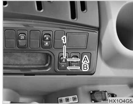
(1) Driving Selection Switch (A) 4WD (B) OFF
