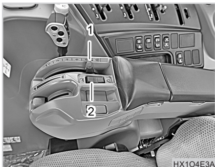
(1) Position Control Lever (2) One-touch Lifting Lever
