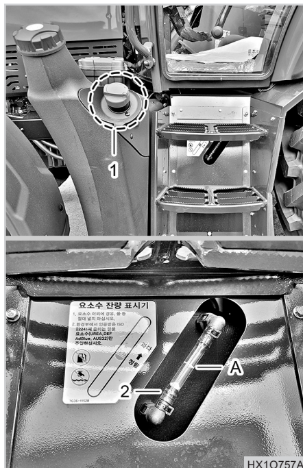
(1) Urea tank (2) Urea level gauge (A) Proper urea level
