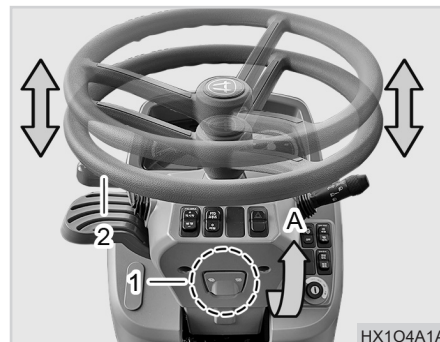
(1) Telescoping Lever (A) Pull
