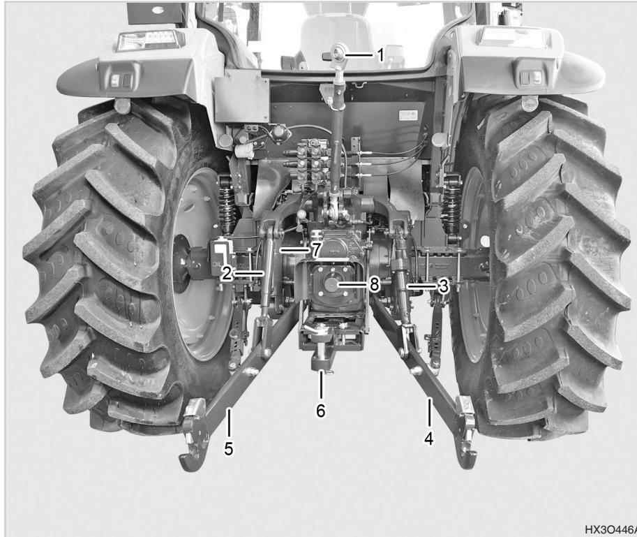
(1) Top Link (2) Lift Rod (L)
