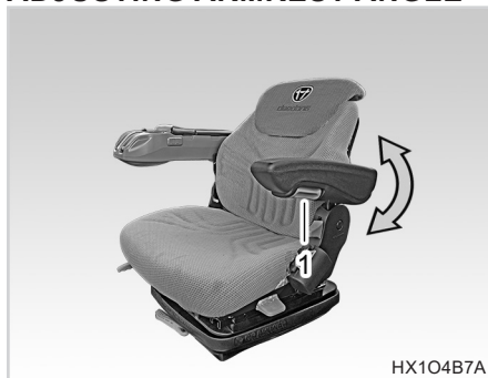
(1) Angle Adjustment Wheel
