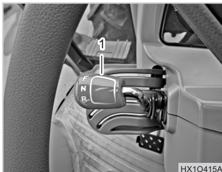
(1) Shuttle Shift Lever (F) Forward (R) Reverse (N) Neutral
