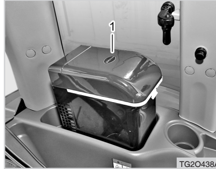
(1) Refrigerator / Heating Cabinet
