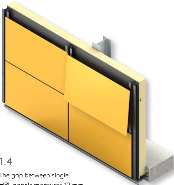
1.2 Vertical KSAL30 Omega (or Z) sections are secured in turn to the Karrier panels using special fasteners. The sections are bedded on PVC sealing tapes. centres between the aluminium sections are given by the HPL module sizes and/or by structural requirements.
