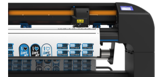
ORANGE status = Lift pinch rollers
