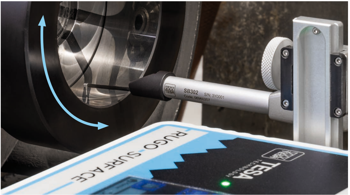
Roughness measurement on a ground adjustment ring mounted on a rotating machine
