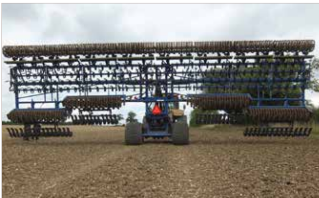
... When fully unfolded, the machine is lowered to the ground.
