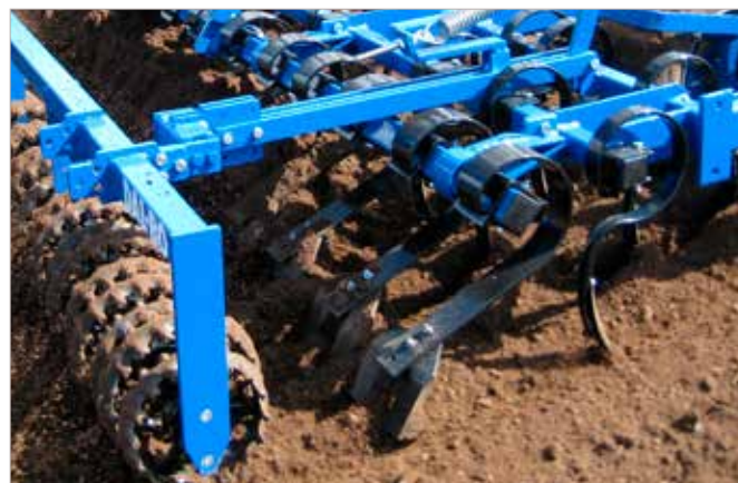
Rear mounted crackerboard
