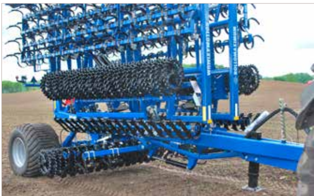
First of all the side sections are lifted clear of the transport
