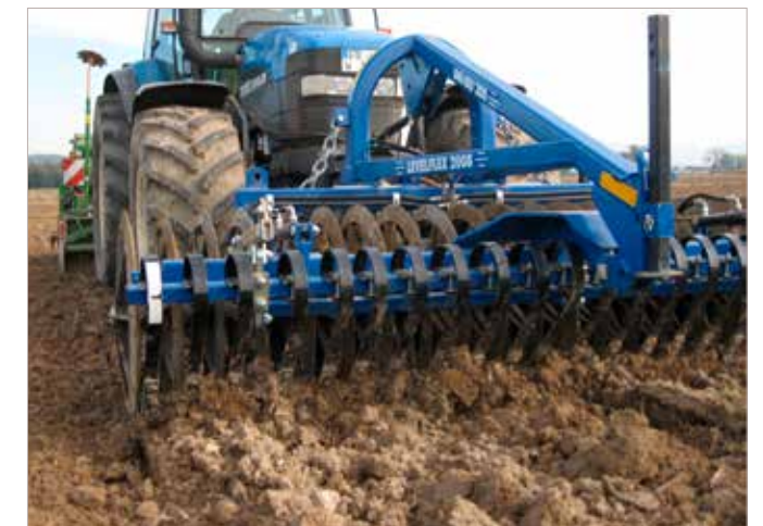
The front mounting and improved geometry actually means that the implement is being 'pulled' forwards, making it easier to steer.
