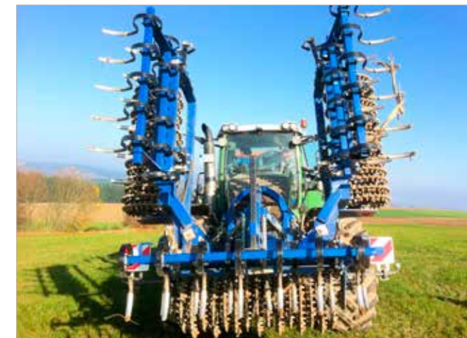
3 m LevelFlex shown with hydraulic cracker board and the Dal-Bo 'V' profile packer
