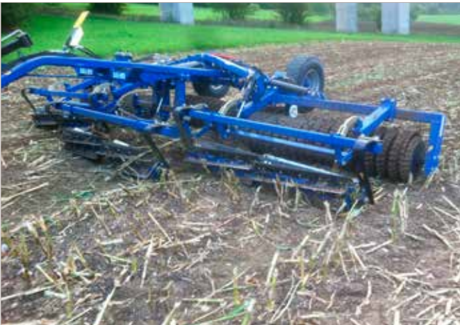
Fitted with a 350mm diameter knife roller
