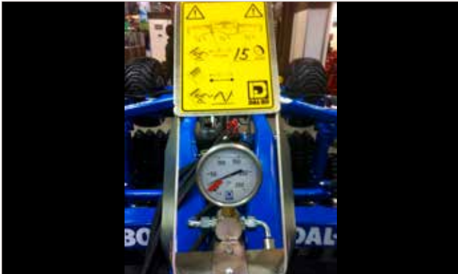
Before using the Maxiroll set the pressure to around 20 bar on the manometer. Put the spool valve into the ‘float’ position and roll!
