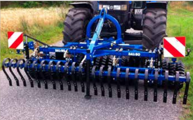
Spindle adjusted crackerboard
