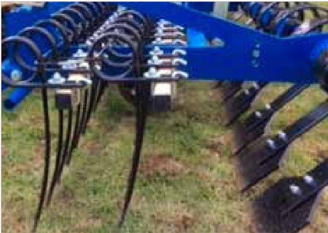
Cracker board and 2 row harrow combination.
