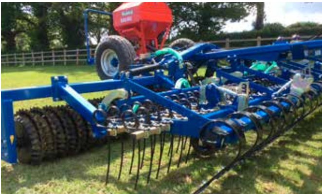
2 rows of harrow tines, cracker board and seeder - one pass solution
