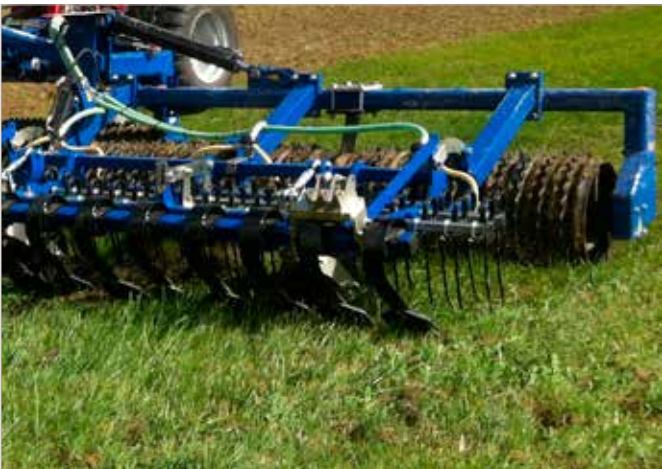
2 rows of 12mm harrow tines in combination with a cracker board
