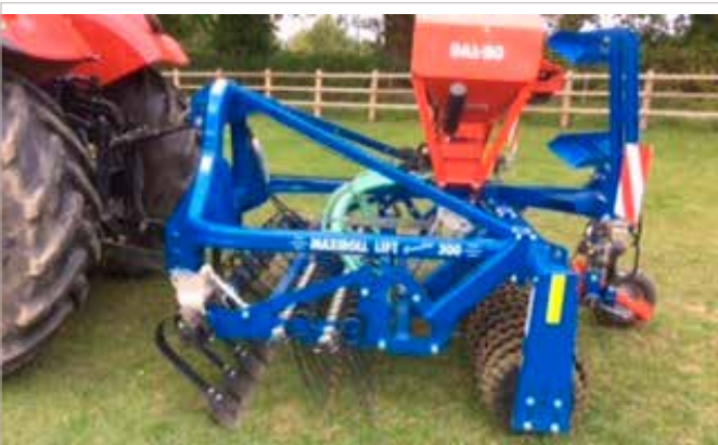
As options Greenline 3 m can be equipped with harrow, cracker board and seeder equipment
