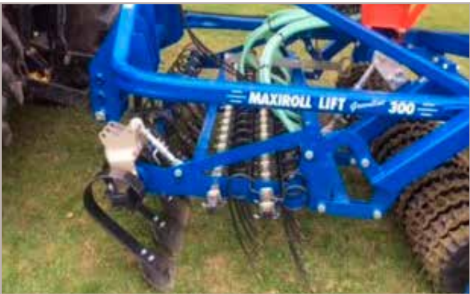
Cracker board with 2 rows of harrow tines
