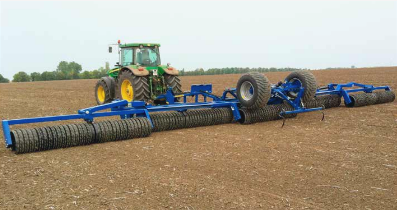
The roller leaves an even and consistent finish across the full working width.
