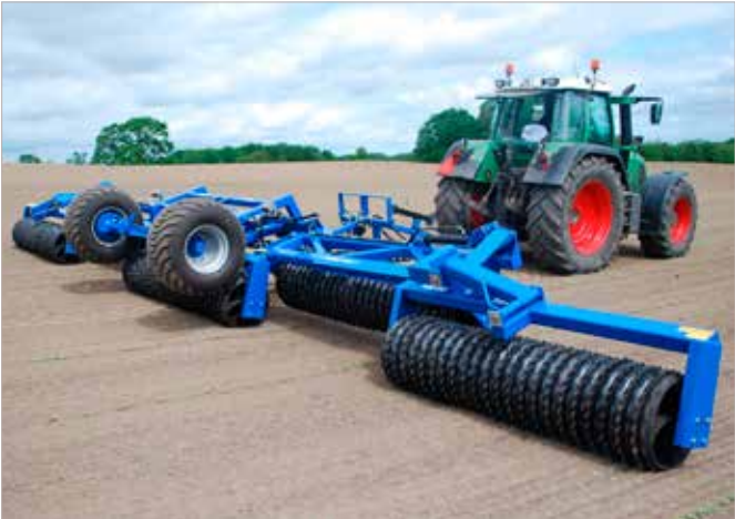
..... as the rolls are lowered to the working position the wheels lift clear of the ground. Now set the pressure in the accumulator(s) to ensure even weight distribution across the full working width of the machine
