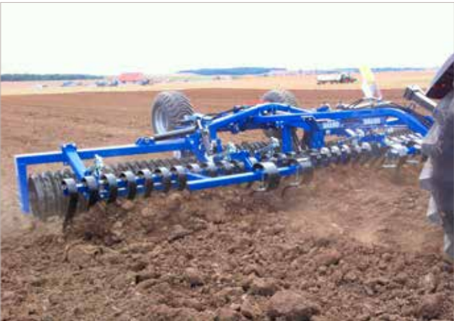
Hydraulically operated cracker board – also fitted with track eradicator tines.
