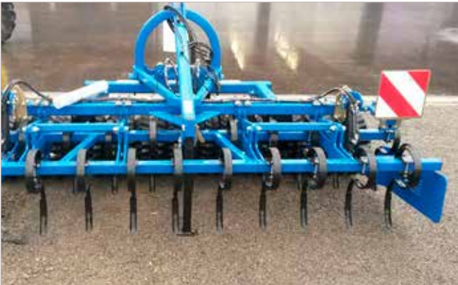
FrontFlex fitted with 2 rows of H/D 45 x 10mm spring tines.
