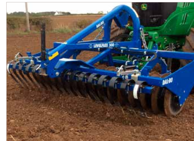
3 m LevelFlex shown with hydraulic cracker board and the Dal-Bo 'V' profile packer
