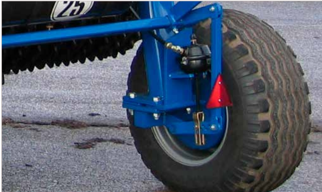
The rollers can be equipped with either hydraulic or air brakes. (Picture: airbrakes)
