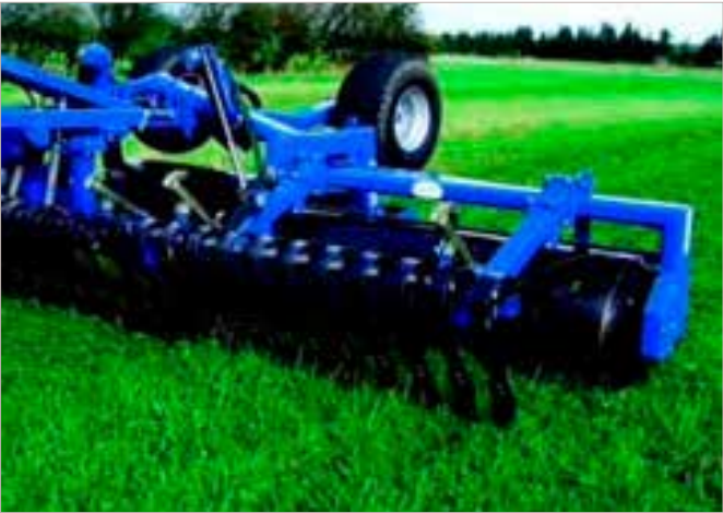
A hydraulic Cracker board can be fitted in front of the roller. The Cracker board is very efficient for preparation and levelling of the ground.
