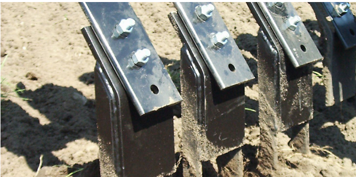
As an alternative to the crackerboard Maxiroll 2008 can be equipped with a 2 row harrow. The angle of the harrow can be adjusted by spindles and the adjustment of the depth is hydraulic.
