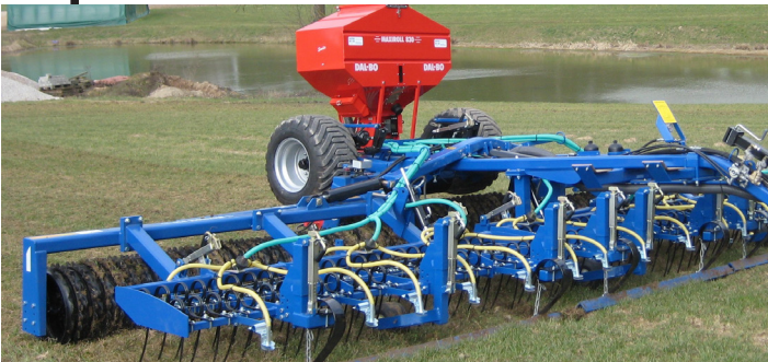
As an alternative to the crackerboard Maxiroll 2008 can be equipped with a 2 row harrow. The angle of the harrow can be adjusted by spindles and the adjustment of the depth is hydraulic.
