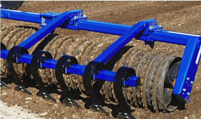
Mounted with hydraulically adjustable cracker board.
