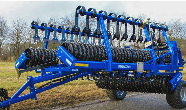
MINIMAX with cracker board, shown here in transport position.
