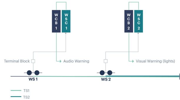
Figure 4: Activation of track warning system with FTVS
