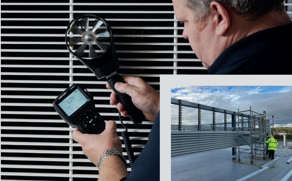
Above: Checking airflow on installed louvre panel. Right: Installation of 1UL/DH louvre.
