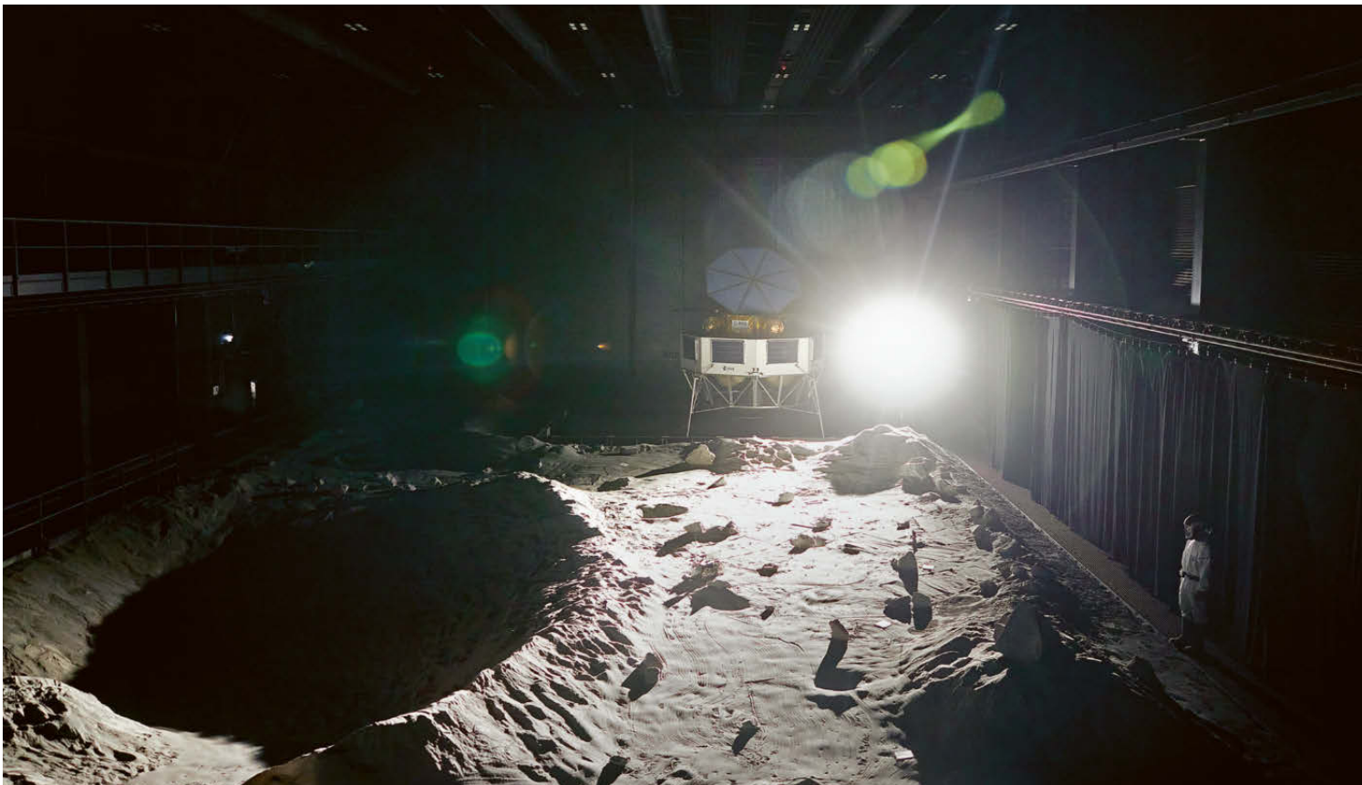
Difficult terrain: The surface of the moon has sharp-edged sand and treacherous shadows, which have been realistically reproduced at the LUNA training facility in Cologne.
