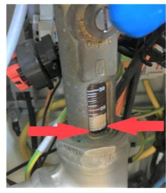
Fig. 61: Flow rate below 10 I/min
