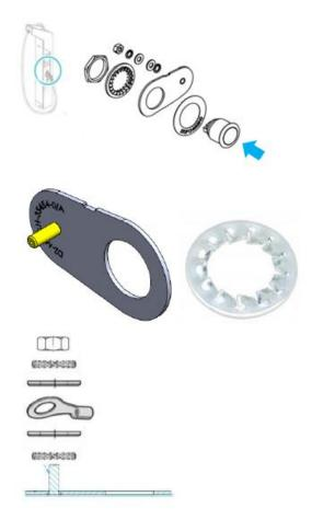
Fig. 231: Charge stop button fixing elements
