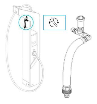
Fig. 133: Upper return, Turbo Charger with closed secondary cooling circuit shown
