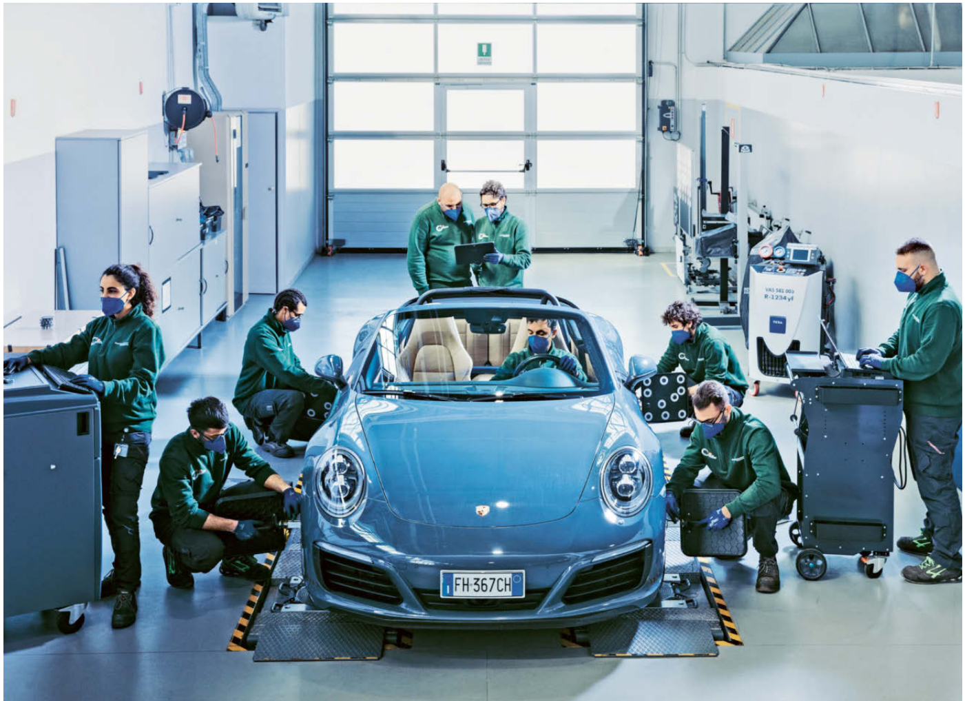
NTC youngsters at work: Up-and-coming mechatronics engineers measure the axles of a test vehicle.
