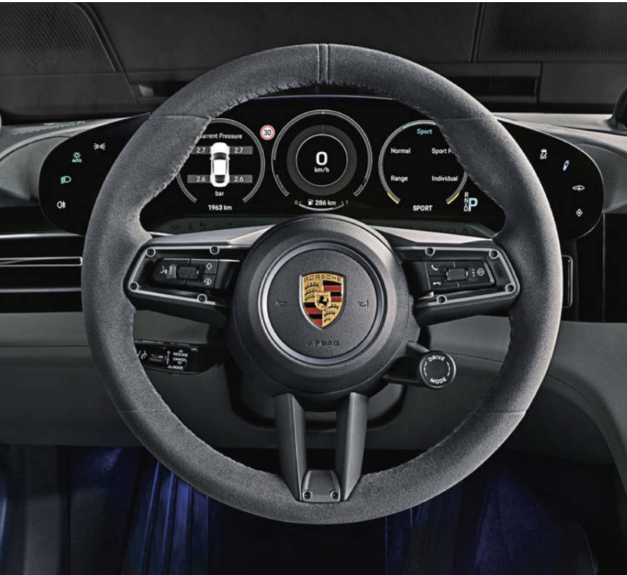
Selection of driving modes: Sport Plus and Sport are especially agile, while Normal and Range optimize the range.
