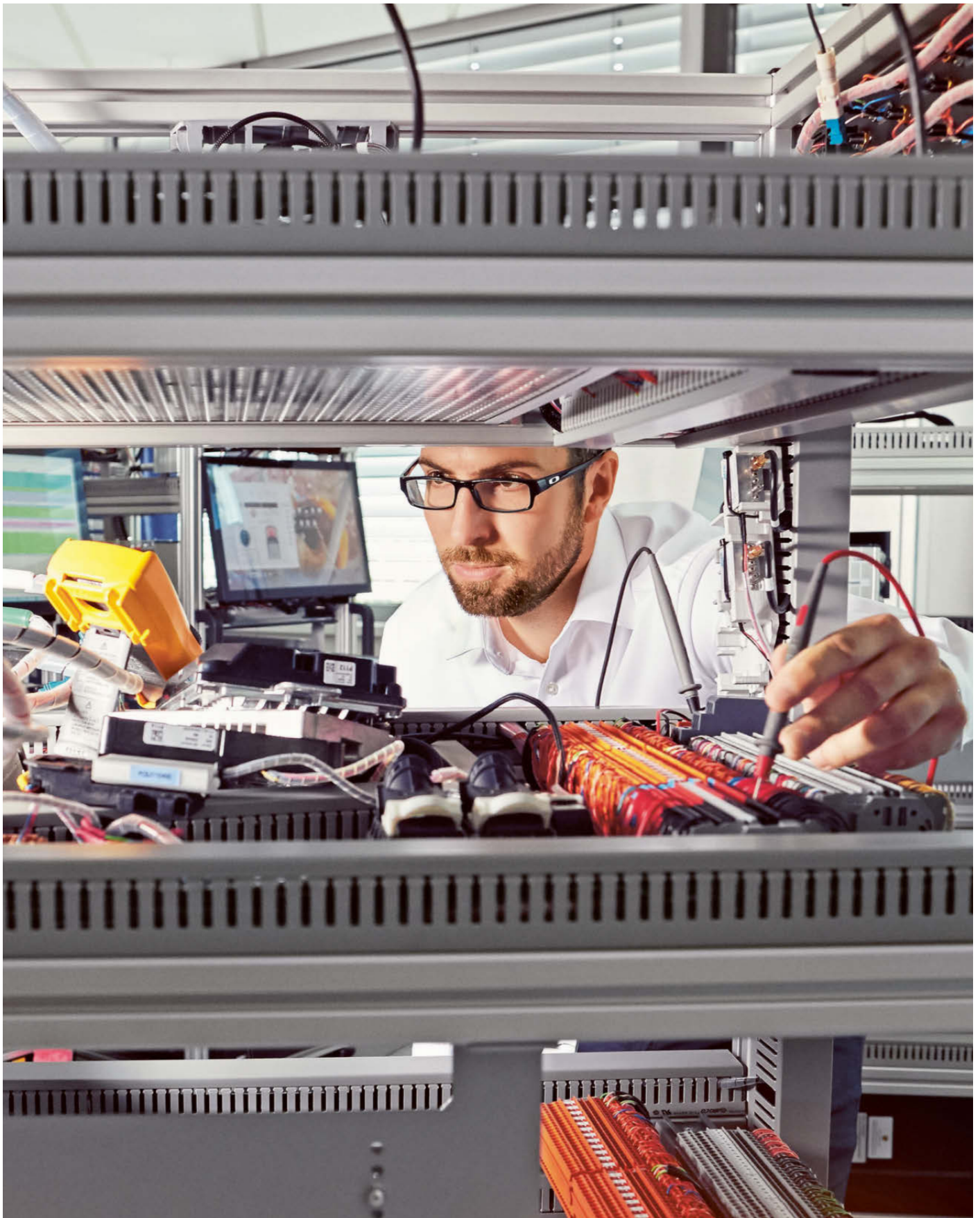
Proven technology: Hardware-in-the-loop is increasingly being used for highly complex systems in addition to component tests.
