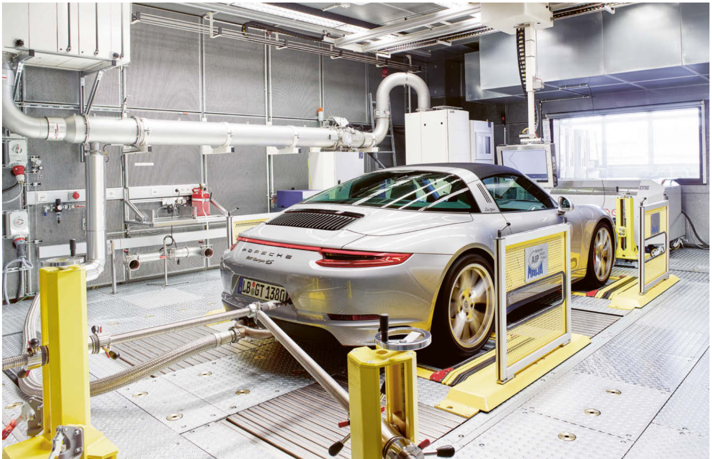
Investigation of emissions-related events: For the type approval tests of a new vehicle model, Porsche Engineering carries out up to 80 test runs on the dynamometer.
