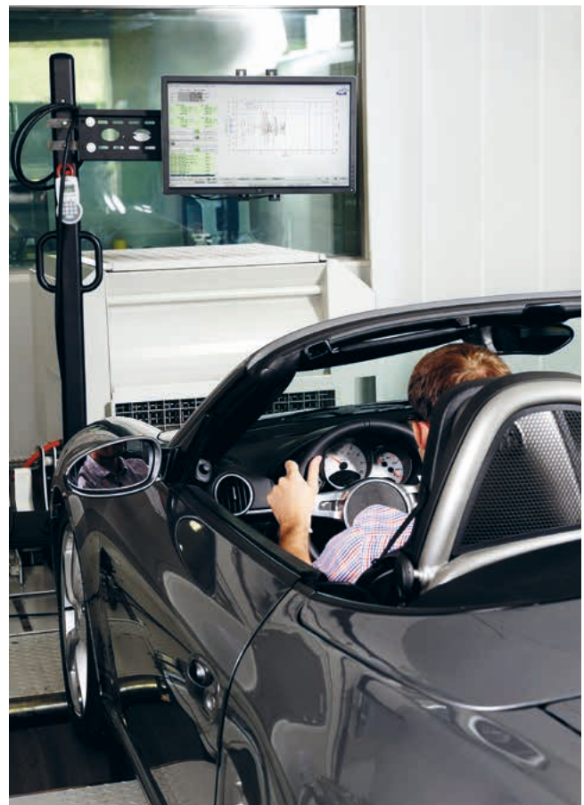
Measurement procedure on the roller test bench
