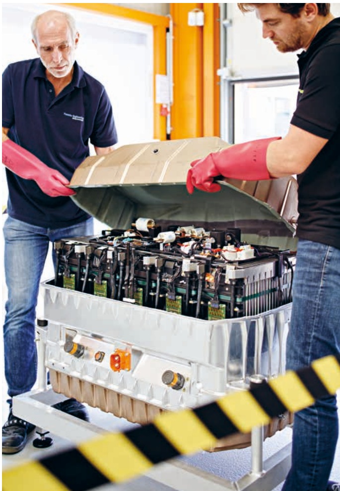
The high-voltage battery for the research project was designed and developed by Porsche Engineering.
