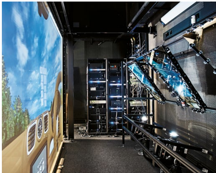
The images are projected from behind onto the screens via high-precision optical mirrors. This avoids objects or people in the interior casting shadows.
