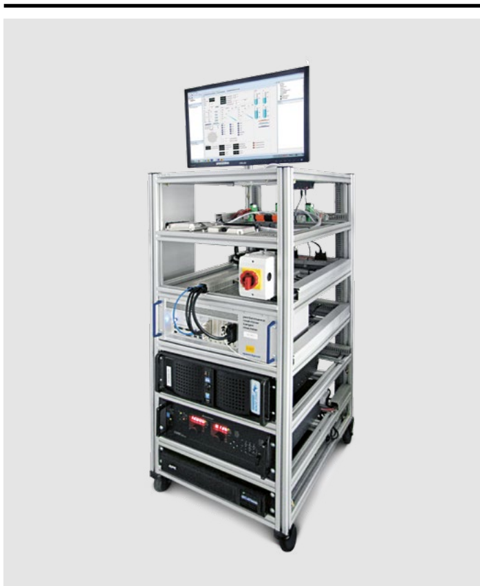
Customized chassis HiL for systems without driver feedback
