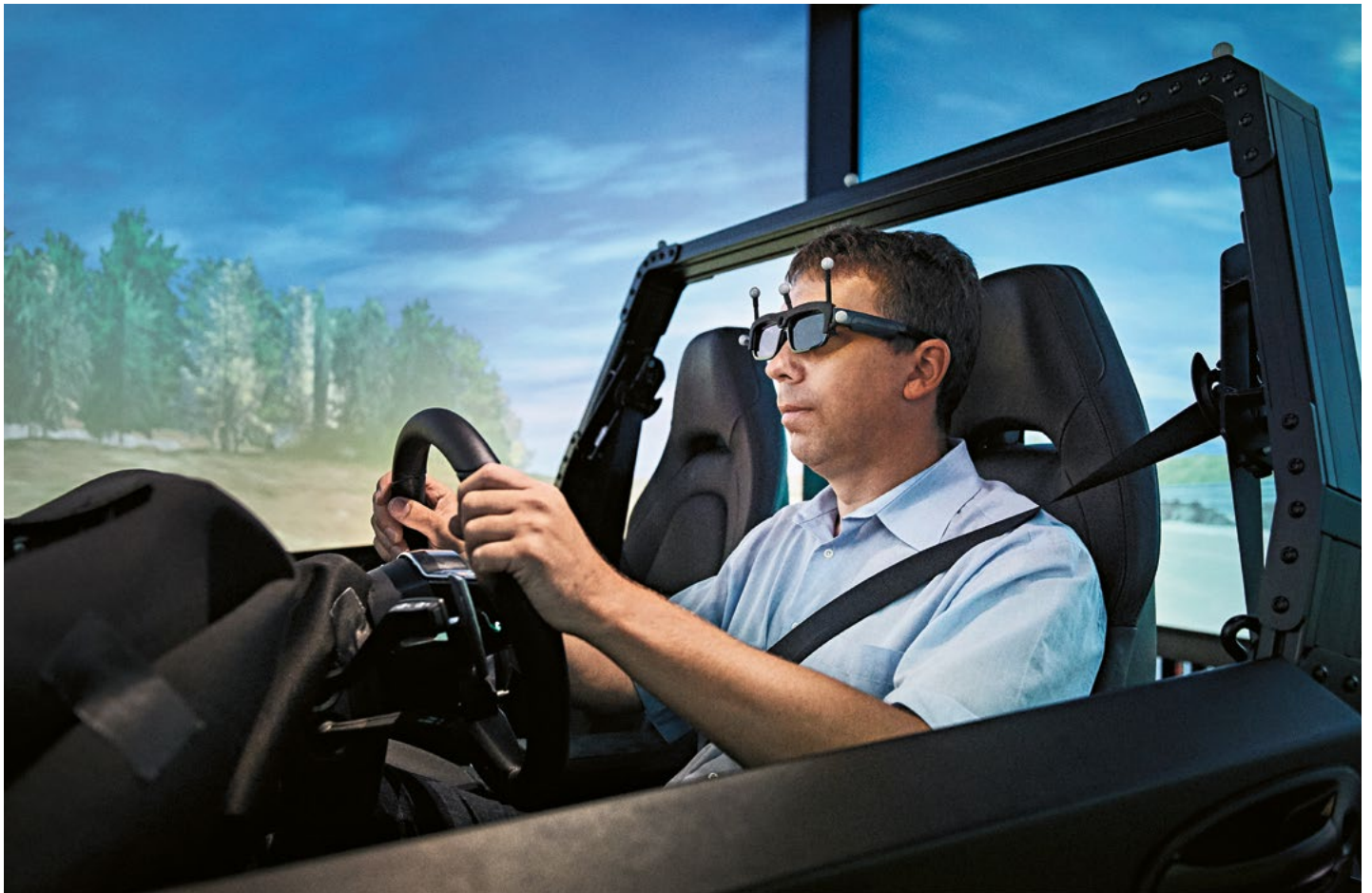
Behind the wheel of a virtual vehicle: The tracked 3D glasses ensure that the driver can perceive the physically correct spatial perspective. Just as when driving “for real”, the driver is wearing his seat belt for safety reasons.
