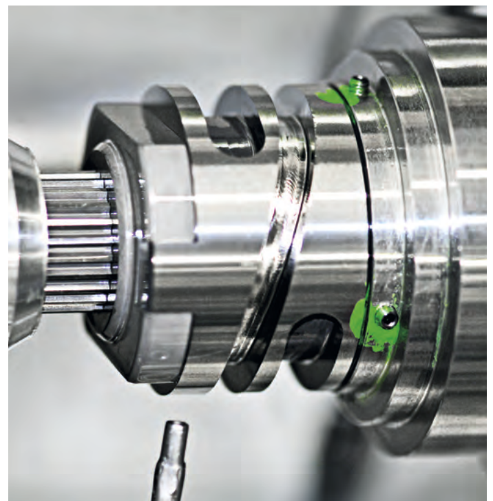
Interchangeable slide piece with endless guide
