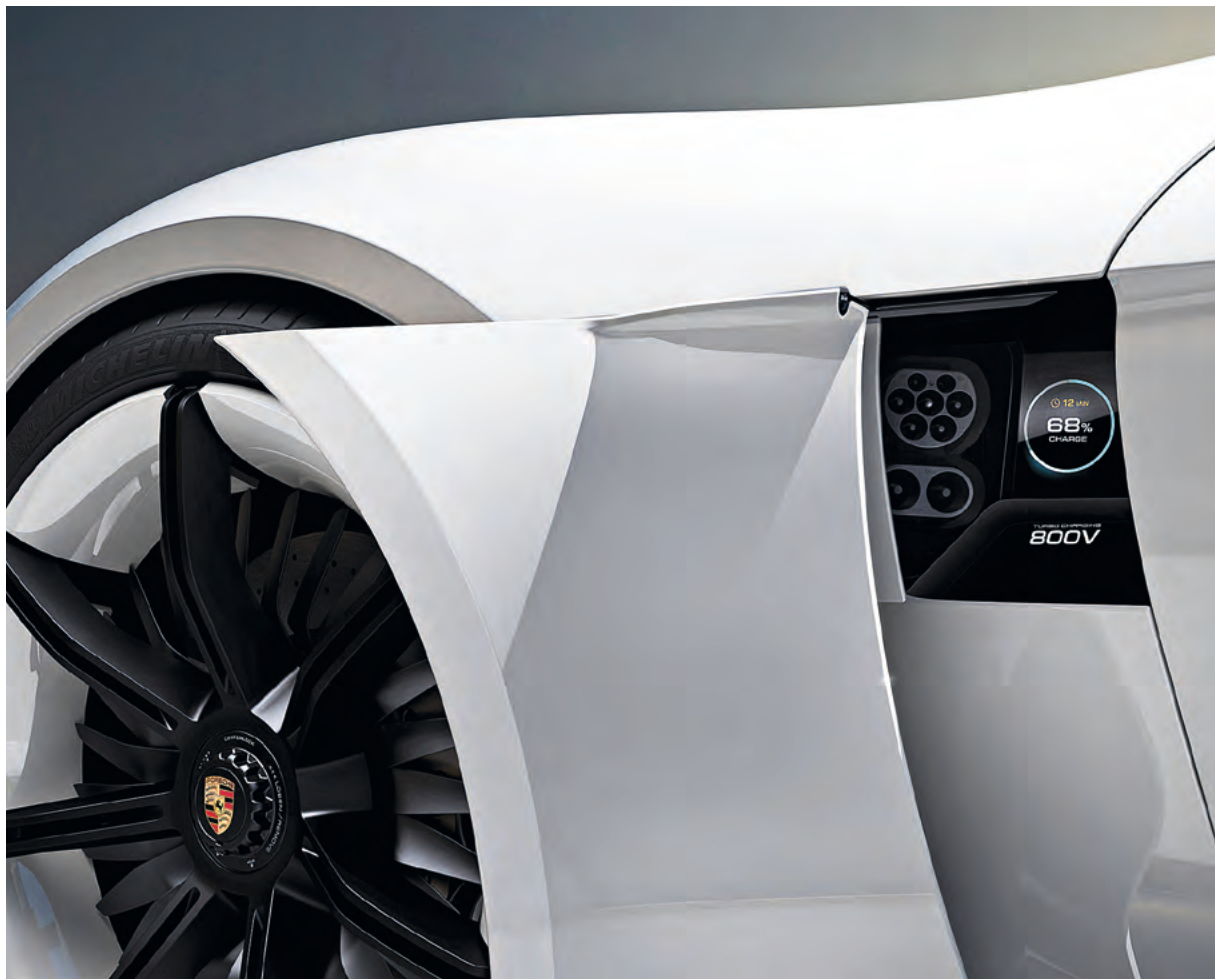
800-volt charging connection on the Porsche Mission E
