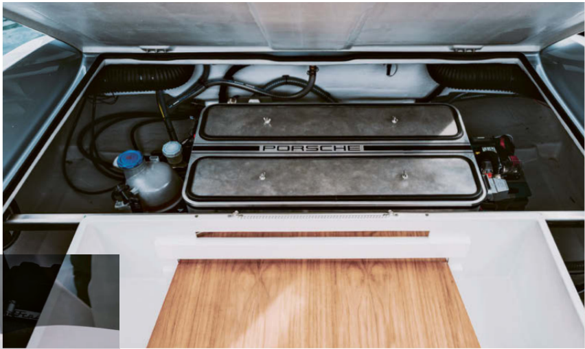
Partners: Michael Frauscher (left in left picture) and Jörg Kerner examine sketches of the eBoat. The lithium-ion battery adopted from the Macan is located under the sun deck in the rear (image on the right).
