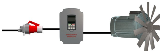
Figure 1: Variable frequency drive (VFD)
