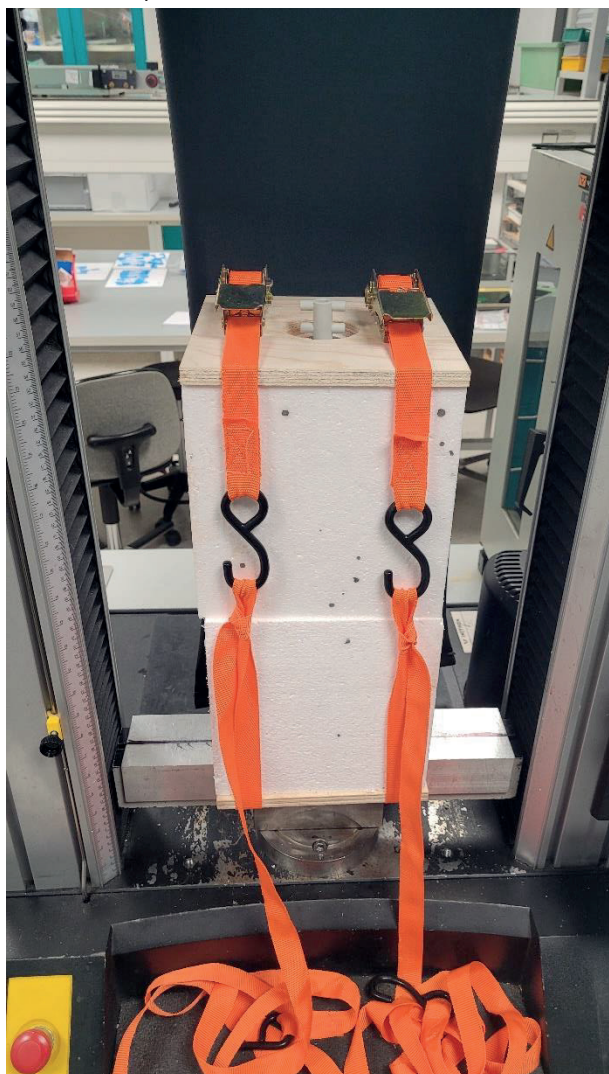
Test setup before extraction of insulation holder
