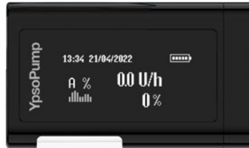
Temporary basal rate on the YpsoPump when in Auto mode
