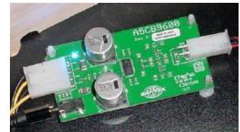
The sound amplifier board is in the front right side of cabinet.
