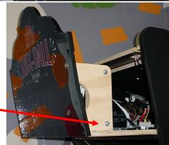
Fold marquee down and re-install the 2 bolts removed earlier. One of the right side, and one on the left side.
