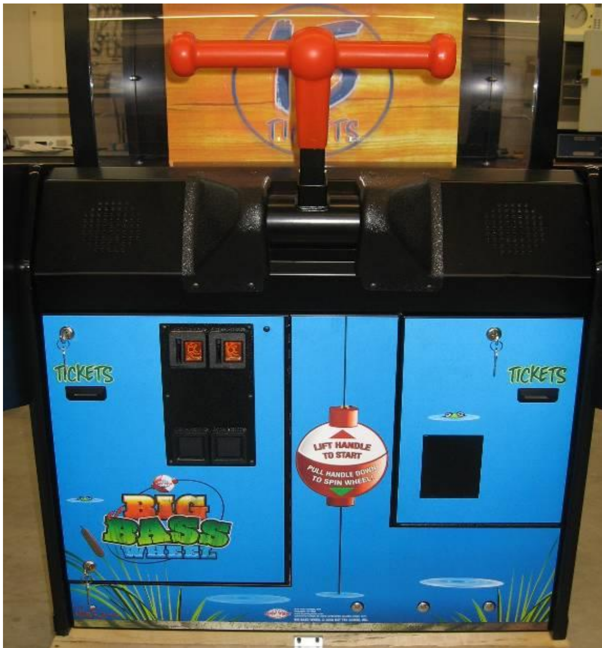
Photo 2 - External view of the Big Bass Wheel showing pull lever, coin collectors and ticket dispensers
