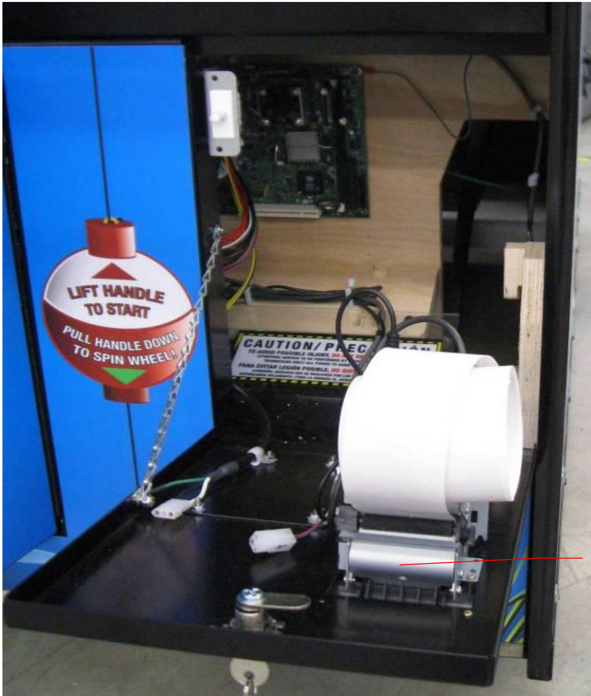
Photo 12 - Internal view of the Big Bass Wheel Pro showing thermal coupon printer and motherboard
