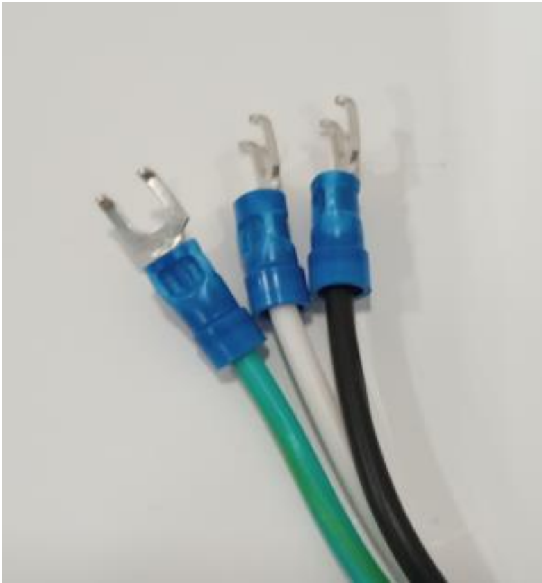
Photo 14 - Locker XL power supply connectors on mains harness, with upturned ends
