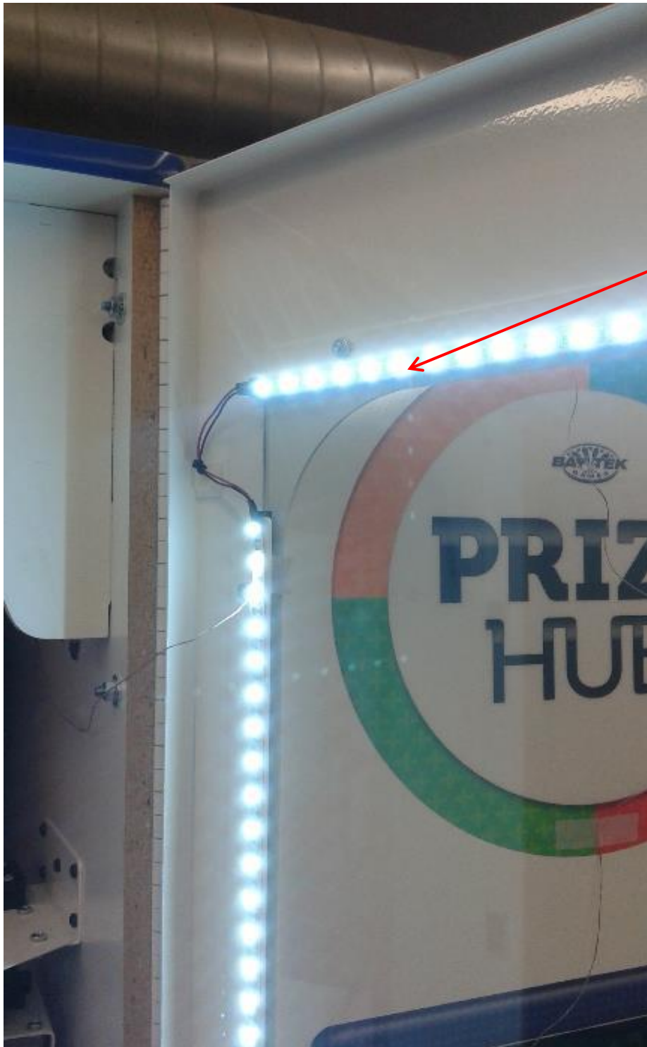
Photo 10 - LED strip inside front door
