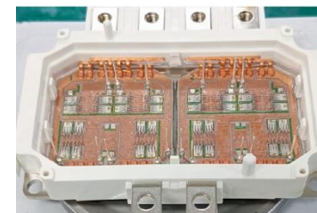
900A SiC half-bridge module
