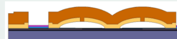
To scale model of a filter cross-section with its thin-film packaging. Credit: CEA-Leti
