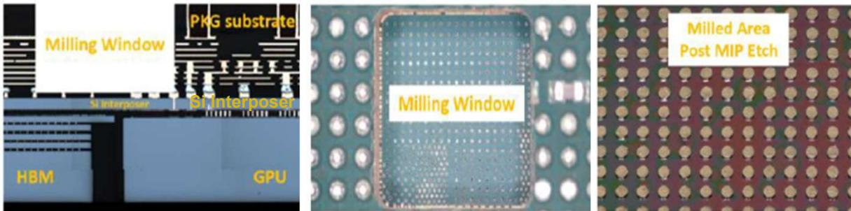
Case Study 1 focuses on the µbump interface between the package substrate and the silicon interposer.
