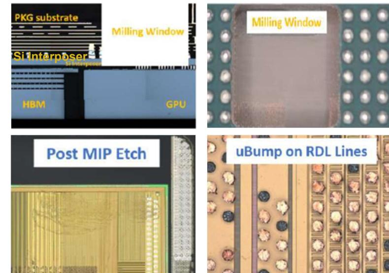
Case Study 2 examines the µbump interface between the silicon interposer and the GPU die
