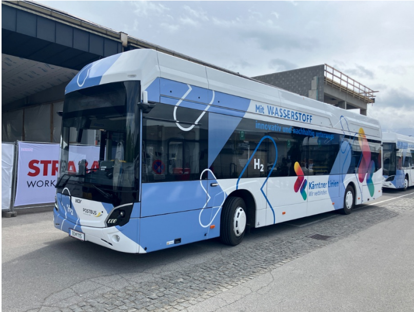
Type MCV C127 FC LE low-floor intercity bus from Österreichische Postbus AG, equipped with VEDS 1.0 electric drive system from Driventic.
