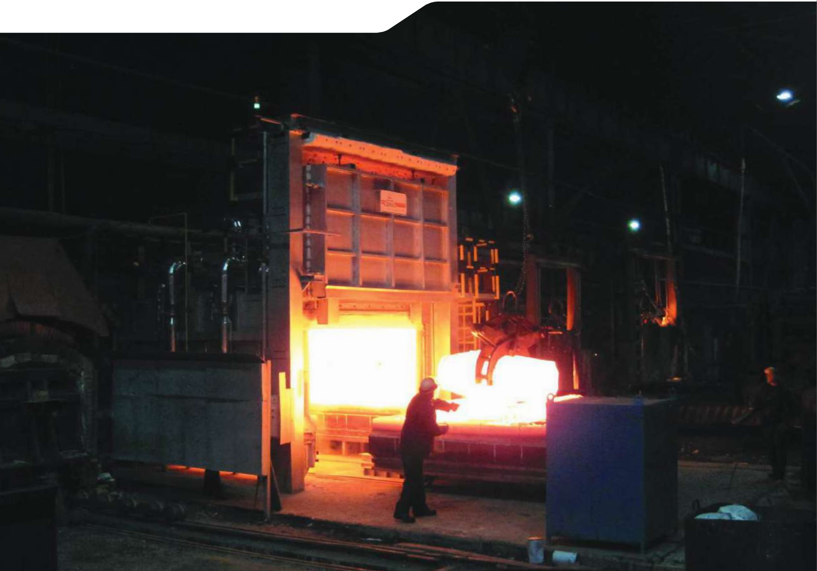
gas heated furnace - 20 m 3 -1300°C
