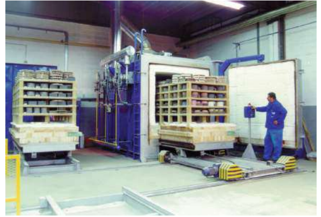
gas heated bogie hearth furnace - 5 m 3 - 1300°C
