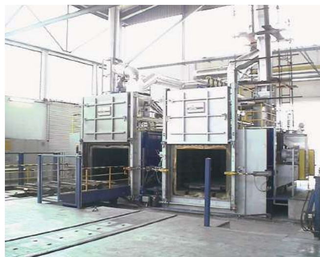
gas heated furnace - 5 tons - 550°C
