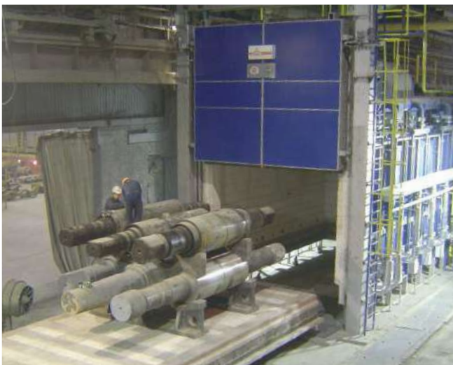
gas heated furnace - 70 m 3 - 1200°C
