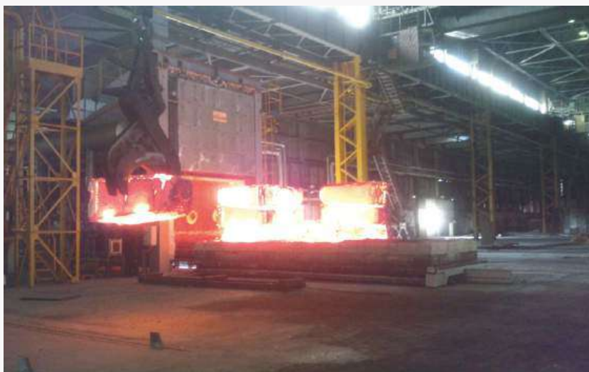
gas heated furnace - 23 m 3 - 1300°C
