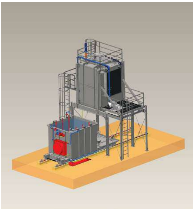
gas heated drop bottom furnace - 4 m 3 - 600°C
