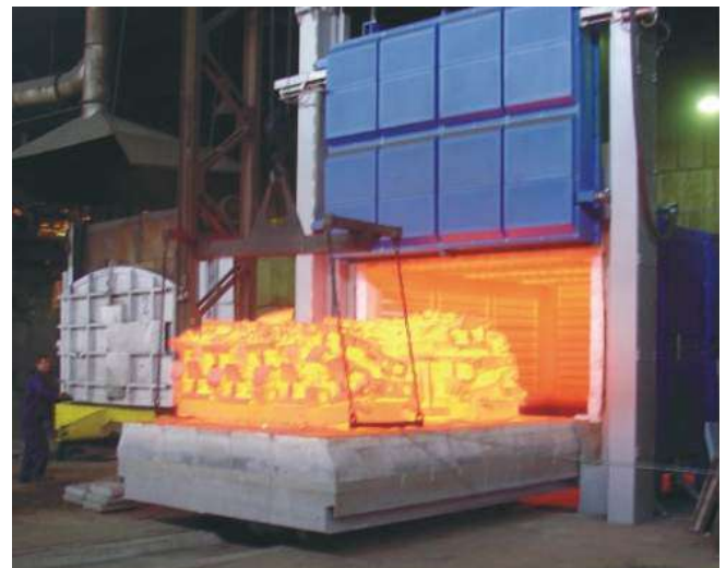
electro heated furnace - 22 m 3 - 1200°C
