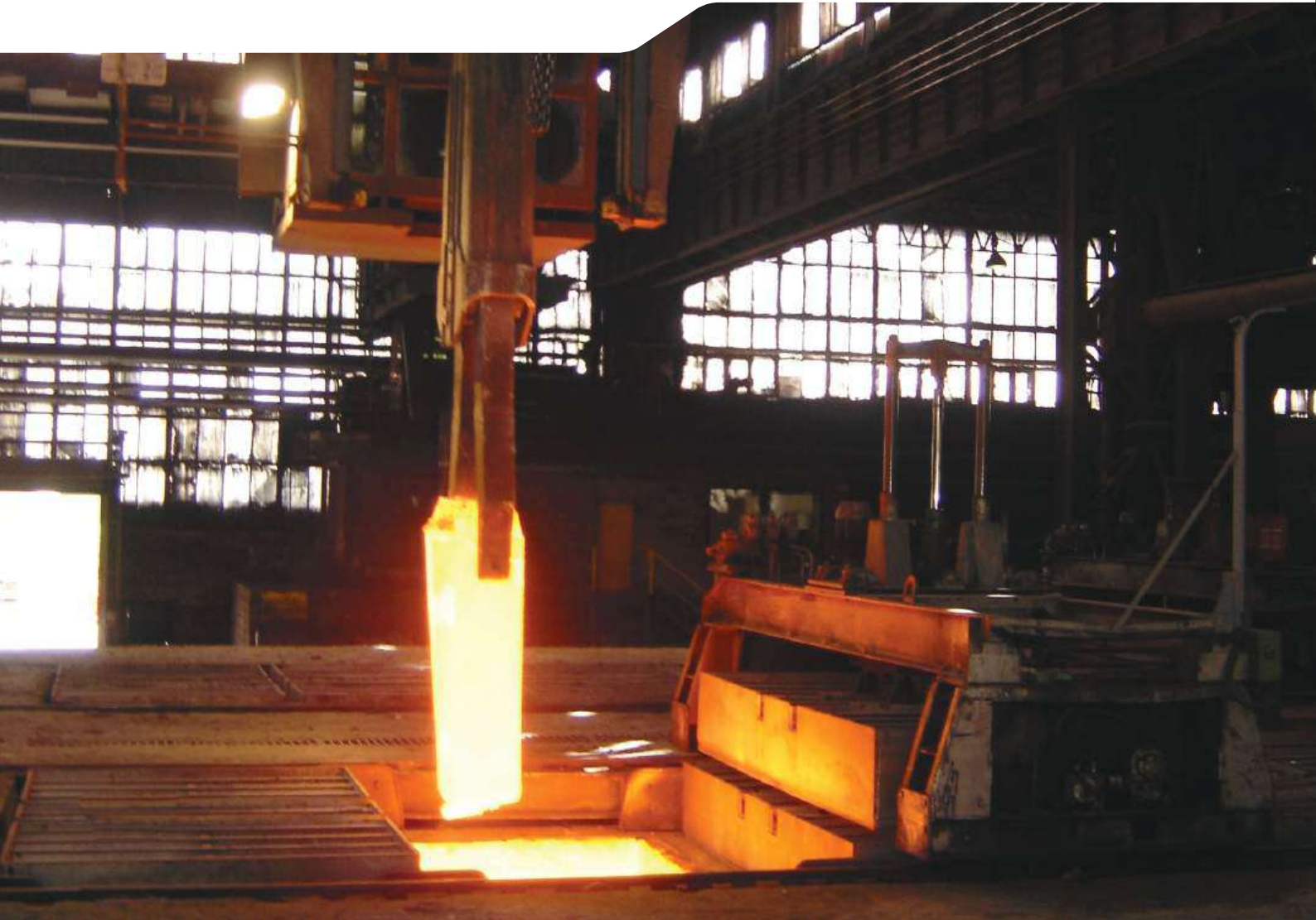
reheating gas heated furnace for ingots
