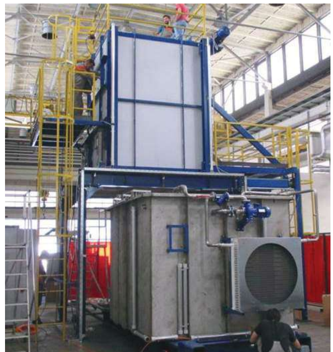
gas heated tilting melting furnace - 1000 kg - 800°C
