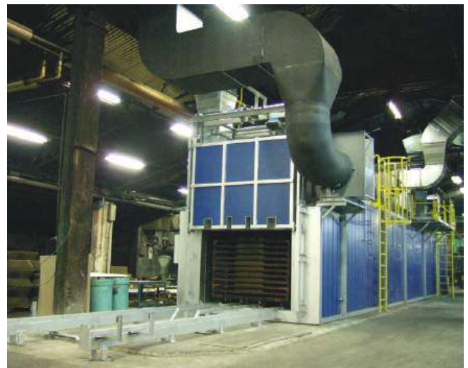
gas heated kiln car conveyor furnace - 600°C
