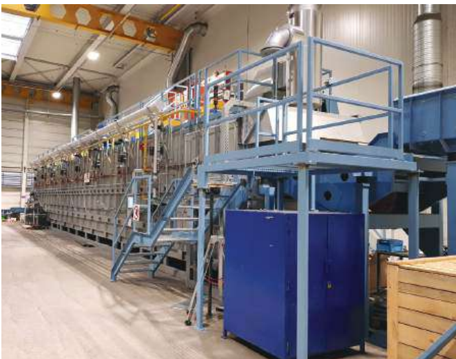
continuous cast link belt furnace – 22 m – 600°C
