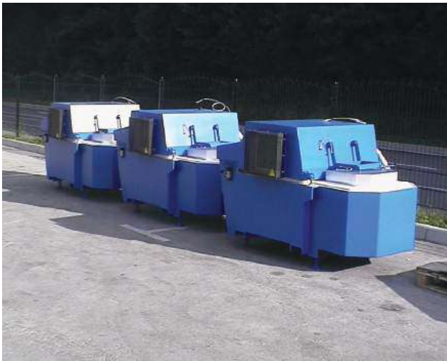
electro heated bath holding furnaces - 1000 kg -
