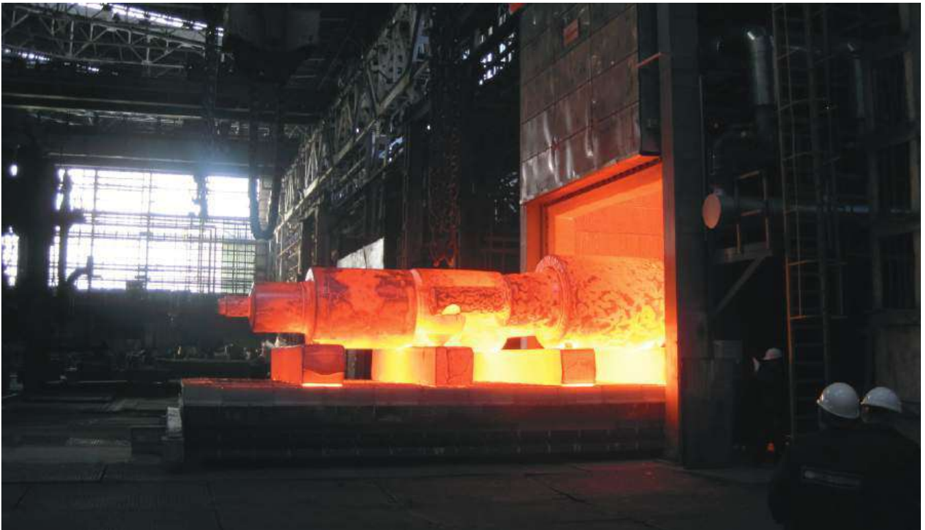
gas heated furnace - 32 m 3 - 1300°C
