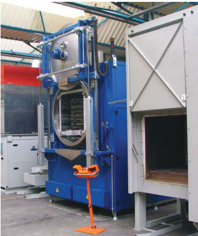
vacuum washing machine with rotating chamber
