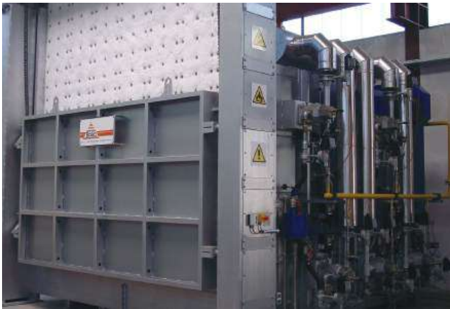
gas heated furnace - 6 m 3 - 1150°C
