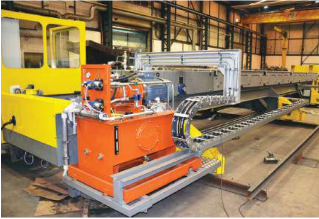
manipulator XYZ - 13 m - 40 tons
