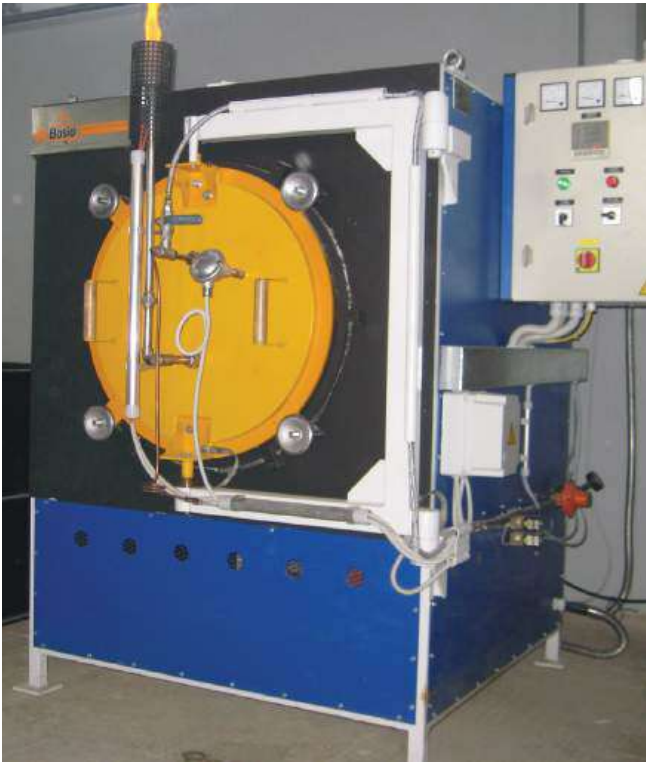
electro heated chamber carburizing furnace - 1000°C
