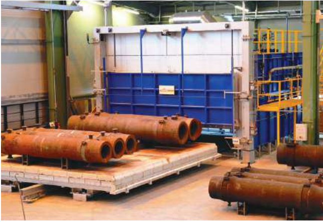
gas heated furnace - 55 m 3 - 450°C
