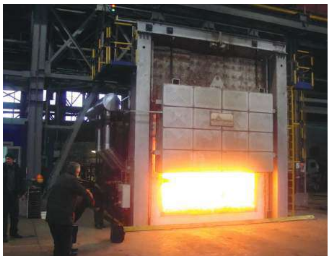
gas heated furnace - 17 m 3 - 1300°C
