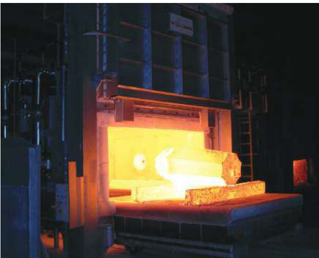
gas heated furnace - 27 m 3 - 1300°C
