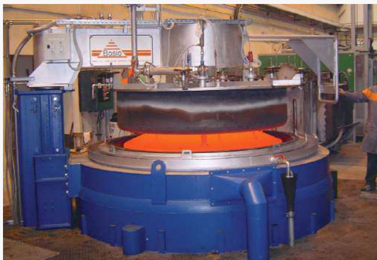
electro heated furnace with controlled atmosphere- 9 m 3 - 950°C
