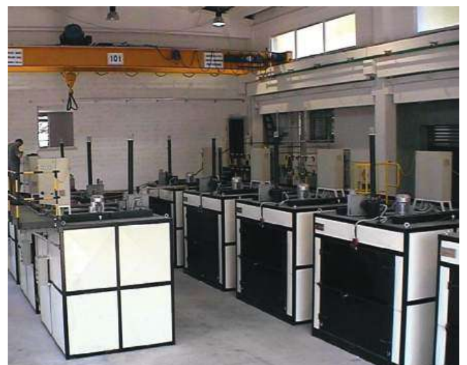
electro heated chamber dryers - 8 m 3 - 250°C
