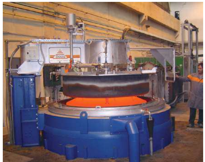
electro heated furnace with controlled atmosphere- 9 m 3 - 950°C
