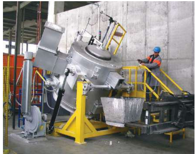
gas heated tilting melting furnace - 1000 kg - 800°C
