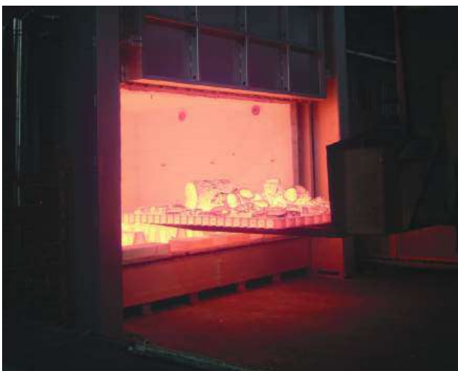
gas heated furnace - 6 m 3 - 1150°C
