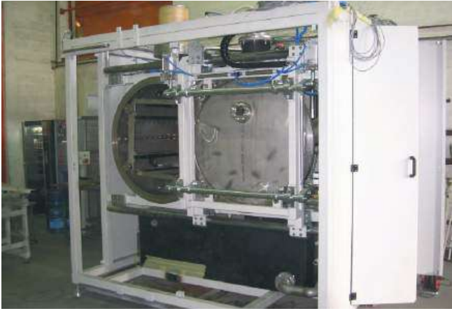
vacuum washing machine with rotating chamber
