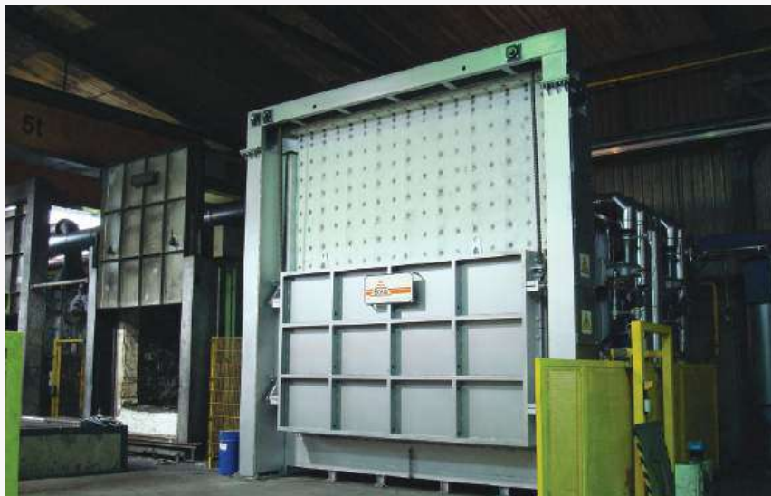
gas heated furnace - 8 m 3 - 1200°C
