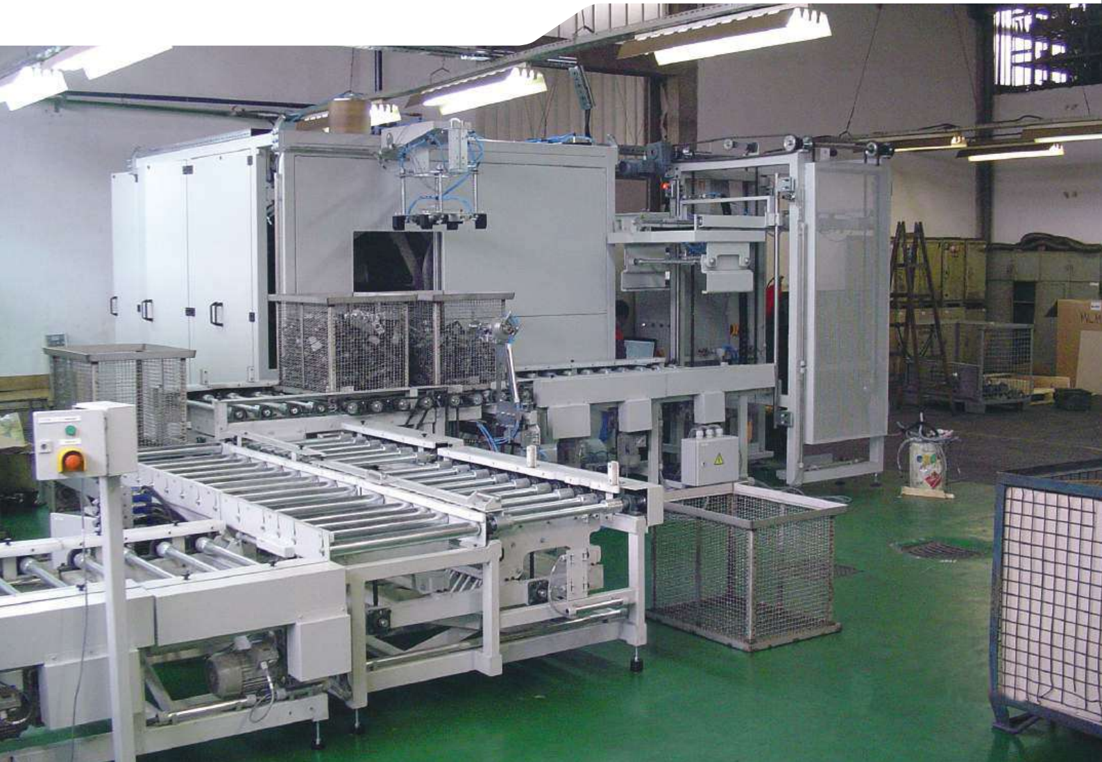
chamber washing machine with transport system
