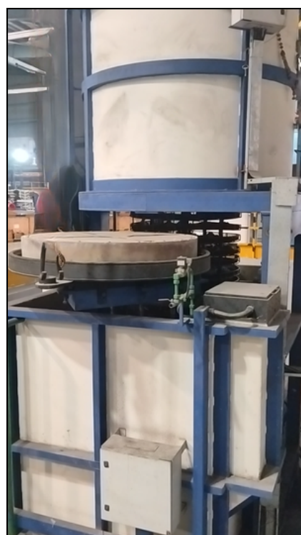
Integrated Quench tank with water heating and agitation.
