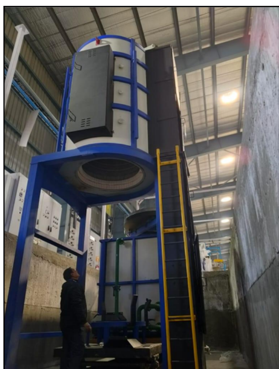
Integrated Quench tank with water heating and agitation.
